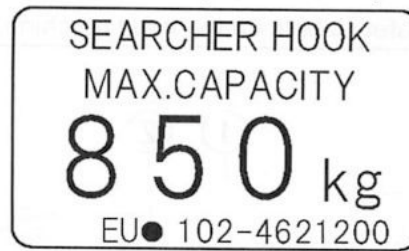
(2) Searcher Hook Maximum Gross Rated Total Load (102-4621200)
