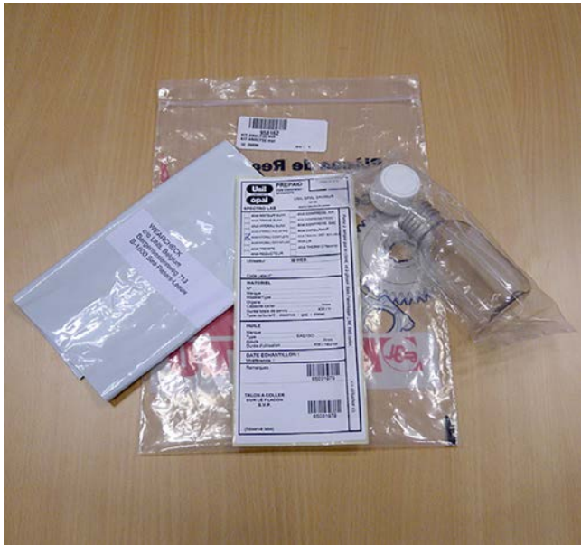
Figure 173: Hydraulic oil contamination check
