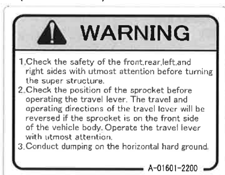
(15) Precautions for swing operation (A-01601-2200)
