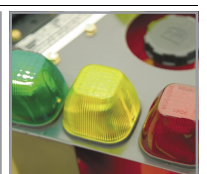
Overload warning lamps + auto stop + alarm
